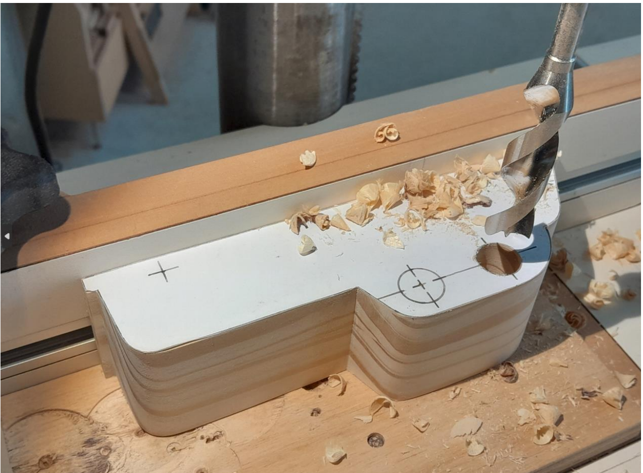
15mm clean cut bit used for the windows.
