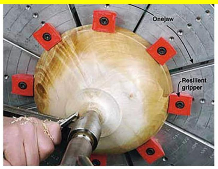
Although each manufacturer has different name for this chuckaccessory, adjustable bowl jaws all work the same. Resilient grippershold the bowl rim to the chuck jaws.
