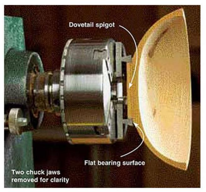
Dovetail jaws contracting around a spigot: When forming a spigot at the bottom of a bowl, match the angle of the outside edge of the spigot to the angle of the jaws.
