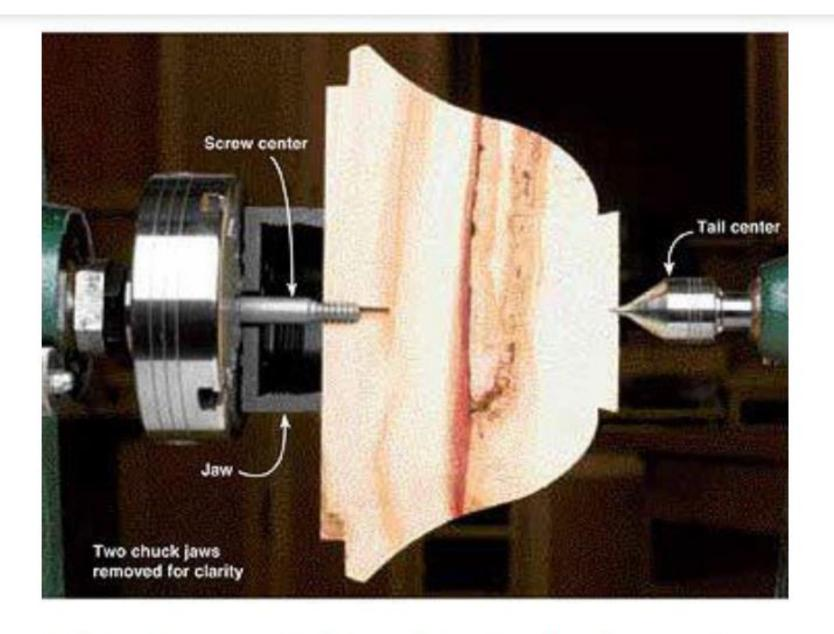
With its exterior shaped, this partiallyformed bowl was cut in half to showhow the screw center secures it to the chuck.
