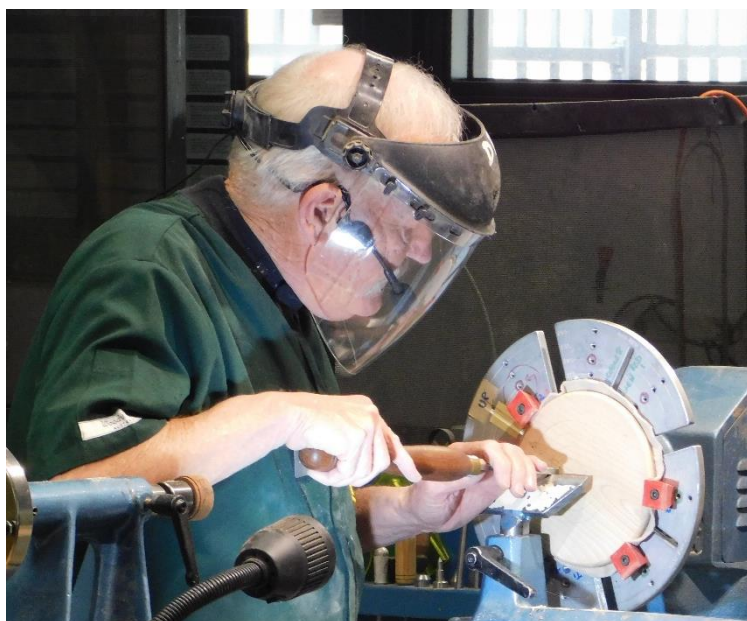
Dave offset turning in Cole Jaws, note position of bumpers.
