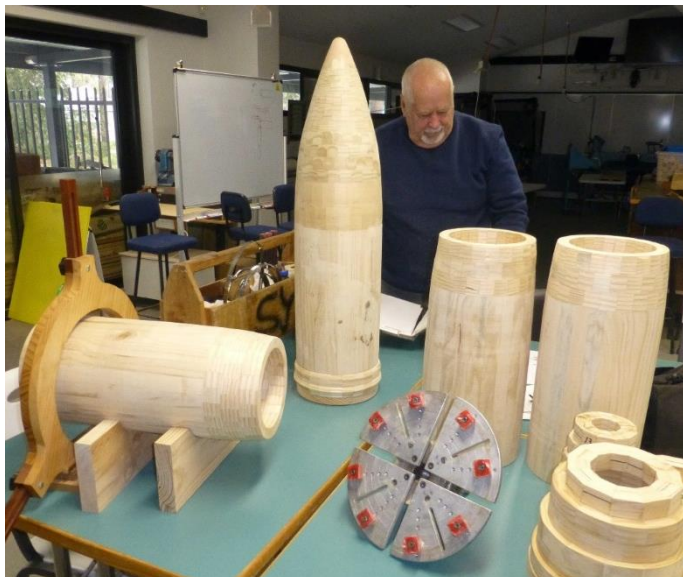
Syd and Ross setting up a shell casing and steady to attach the projectile for final shaping.
