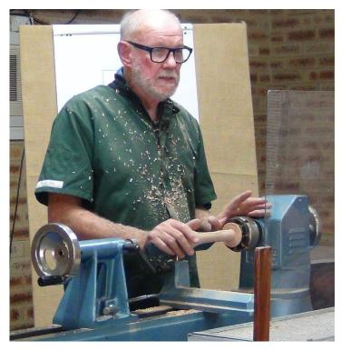
Then cut it in halves with a spigot on both ends of each piece, so he had a grain match for the top and bottom section of the grinder. He then placed the bottom section in the chuck with the top to the tail stock and proceed to drill holes to suit the internal measurement of the grinder 30 mm forstner bit first then a 25mm auger bit making sure he did not go too far, then reversed the blank in the chuck to drill a 45mm hole 20mm deep then a 38 mm hole as deep as
