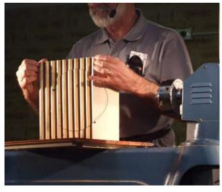
Andy showed previously glued up piece with a bowl shaped marked and cut out on a bandsaw. The blank was mounted in a chuck and a bowl turned in the conventual manner.
