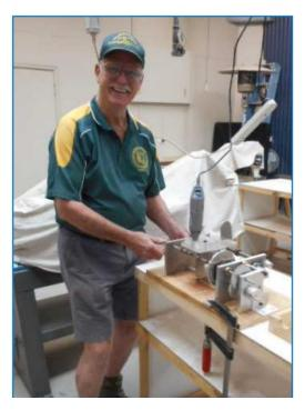
This interesting contraption has been built from scratch by John. It uses a Dremel as a router to cut enhancements and is suitable for small cylindrical items such as pens. It's inbuilt indexing coupled with an adjustable drive gearing mechanism produces various types of enhancement. A possible future attachment would be a pyrography pen to burn patterns.
