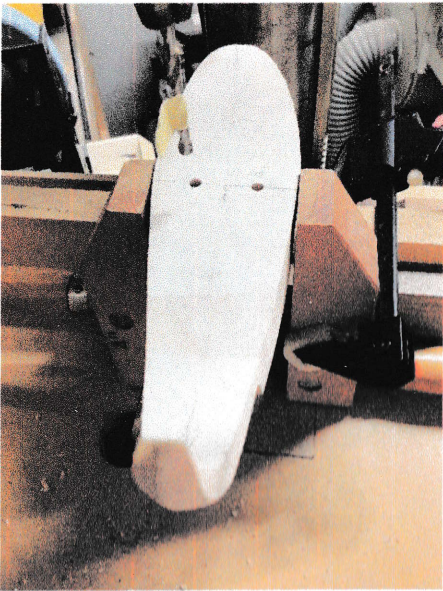
7) Mark and drill two 4mm holes for legs of ibis.
