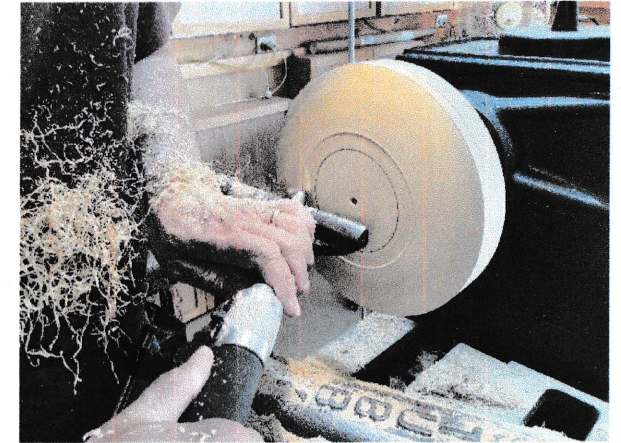
3) Turn a convex shape towards the centre line. Sand and finish.
