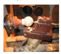
As can be seen from the photograph, I have used the stem of a tool rest as pivot, the exact centre of which must be positioned directly under the centre of the ball – *locked* in position and not moved for any adjustment.
