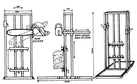
NOTE: SLIDES 'A' AND 'B' — SAW GUIDE BAR AND LOG JAWS ARE CUT FROM 30 MM X 30 MM R HS — RIGHT ANGLED LOCKING BOLTS ARE REQUIRED ON ALL SLIDES.
