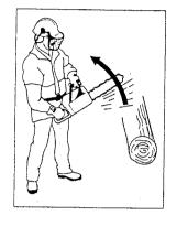
Kickback can happen very suddenly and violently; kicking the saw, bar and chain back at the user. If this happens when the chain is moving it can cause very serious, even fatal injuries. It is vital you understand what causes kickback and that you can avoid it by taking care and using the right work technique.
