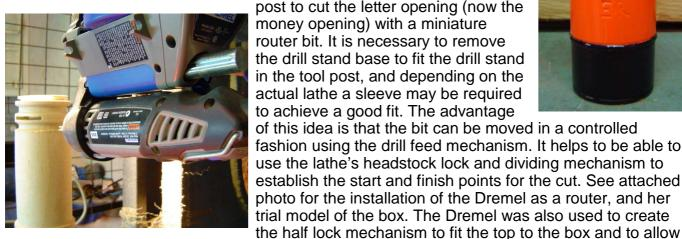
post to cut the letter opening (now the money opening) with a miniature router bit. It is necessary to remove the drill stand base to fit the drill stand in the tool post, and depending on the actual lathe a sleeve may be required to achieve a good fit. The advantage
