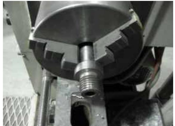
Mandrel in a metal lathe ready to accept a manufactured faceplate to be trued up.
