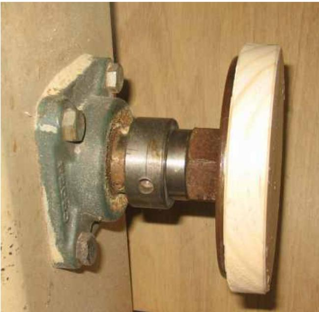
In the above photo, there is a spacer between the head stock end the nut of the faceplate-this is a must when the nut does not seat up against the head stock.
