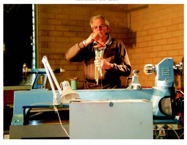
First he made the top from which the chimes are to hang, Viv used a template to mark the position to drill holes for the cords in the blank, after mounting between chuck and live centre he cut a spigot which he fastened in the chuck to cut another spigot for the bottom he then shaped, sanded and finished. Viv then reversed the piece and shaped the top and sides, sanded and finished.
