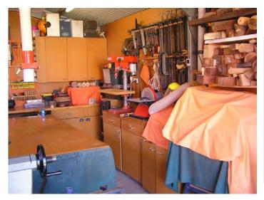
Plate 4: The northern wall, showing successively from left to right a drill stand and sander mounted on mobile equipment cupboards, a router table (covered) on a cupboard containing a thicknesser, and a table saw, also covered on which is placed a Rose engine. Part of the timber rack is on show above the Rose engine while, at the other end, is a rack for clamps of varying types. In the right-hand corner of the workbench is a microwave, also covered.
