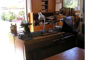
Plate 2: Looking towards the door, showing the cupboard/workbench on the eastern wall. The structure of the lathe stand is evident. Note also the mobile tool trolley at the right hand end of the lathe.
