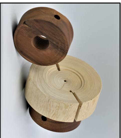
A glue chuck, and a glue chuck with a sacrificial block adhered to the chuck. The slots in the sacrificial block allow access close to the bottom of a bowl when using callipers to measure bowl thickness.
