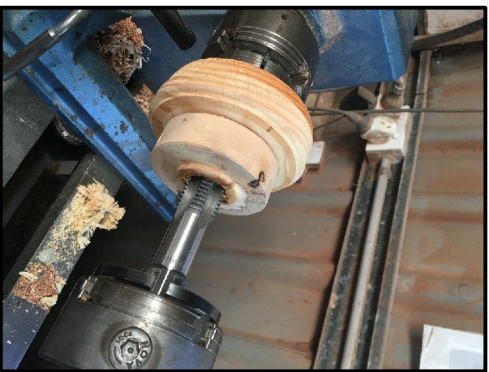
A glue chuck being tapped by Ted Stewart-Wynne. Ted is using a chuck mounted on the lathe tail-stock to hold the threading tap.
