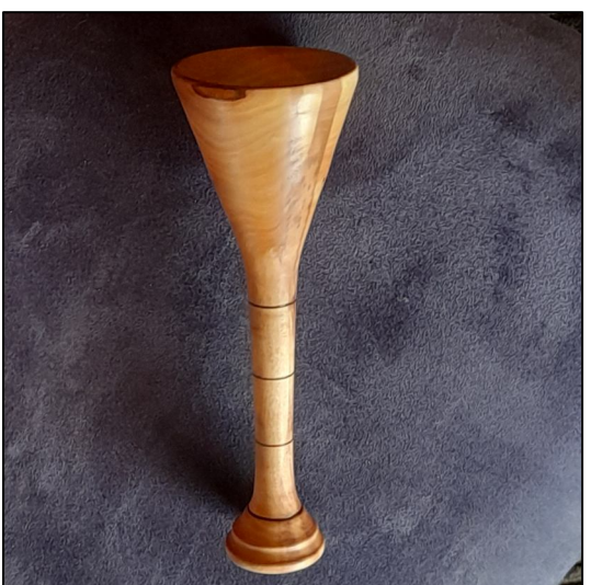
A Pinard Stethoscope turned by Neil George in olive and finished with Livos oil.
