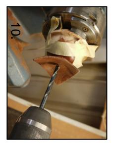
Once finished and sanded and while still take the spigot of the top finial. taped to the jam chuck, drill a 6mm hole to
