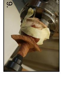
of the wing to same thickness as the first as possible for strength. Shape the inside with the help of some hot melt glue and Now reverse the star onto the jam chuck it up, again leaving the spigot on as long tape. Use the live cone centre to help line
