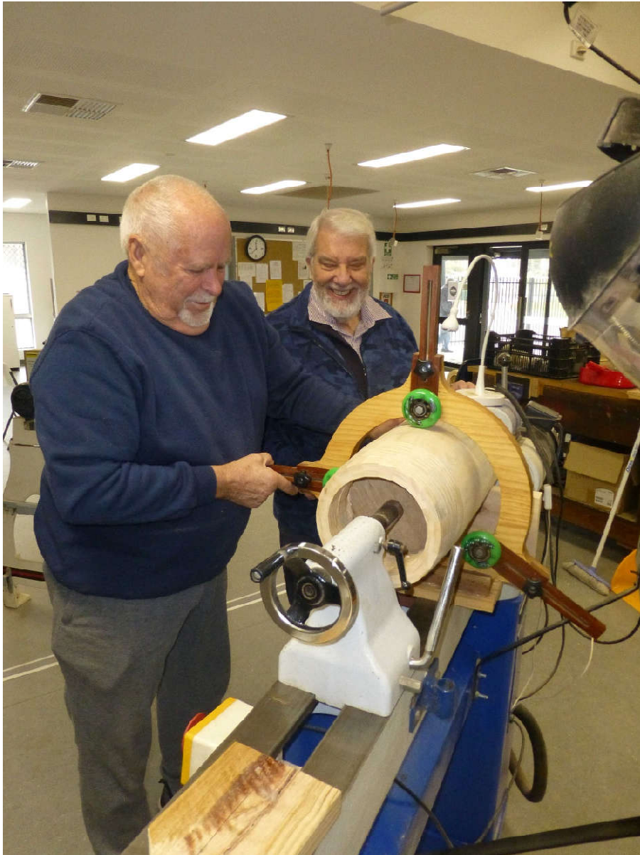
Syd and Ross setting up a shell casing and steady to attach the projectile for final shaping.
