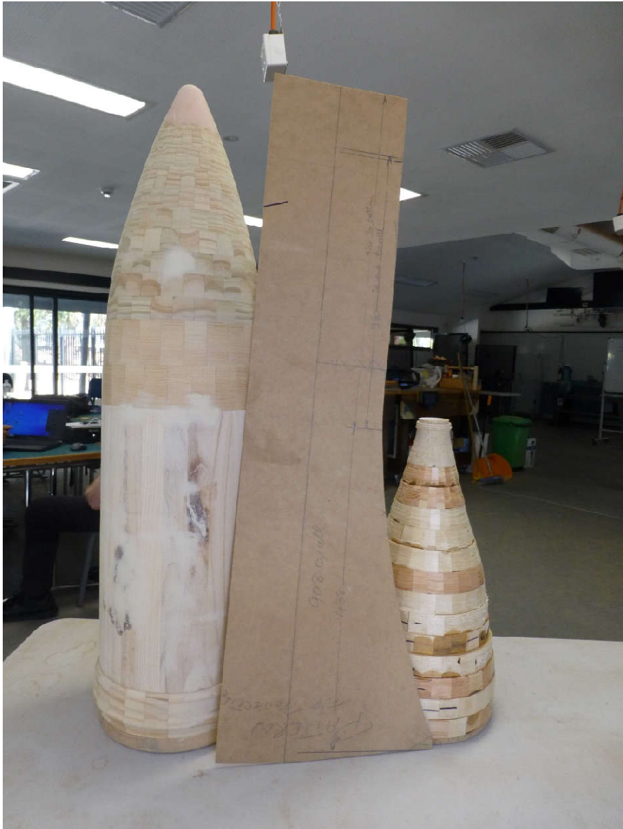
Syd's finished shell, the template he made for shaping and Aiton's roughly turned projectile.
