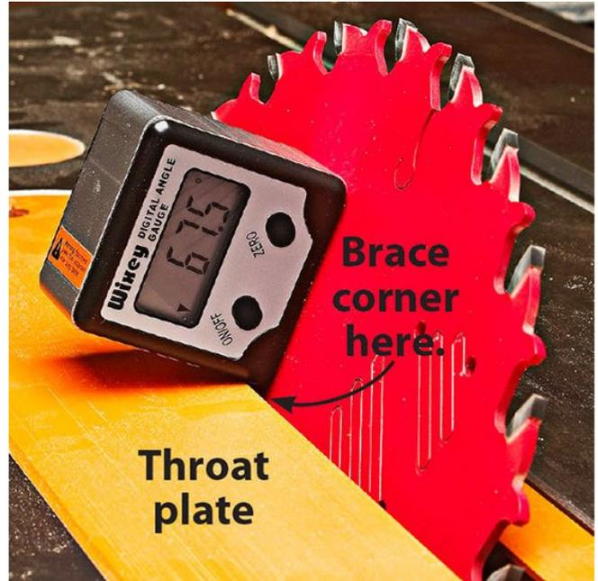
Brace an electronic angle gauge against the throat plate so it doesn't accidentally rotate and produce a false reading.
