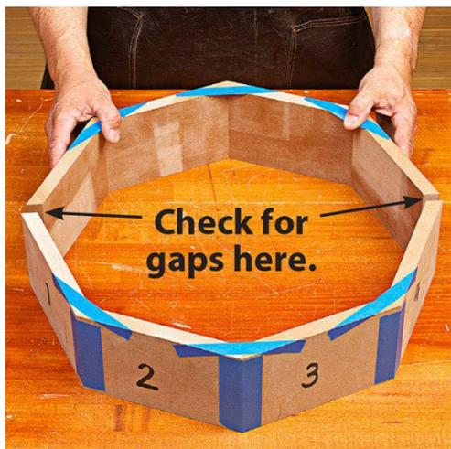
Tape two halves made from test scraps; then butt the halves together to see where gaps develop. Avoid flexing the two halves.
